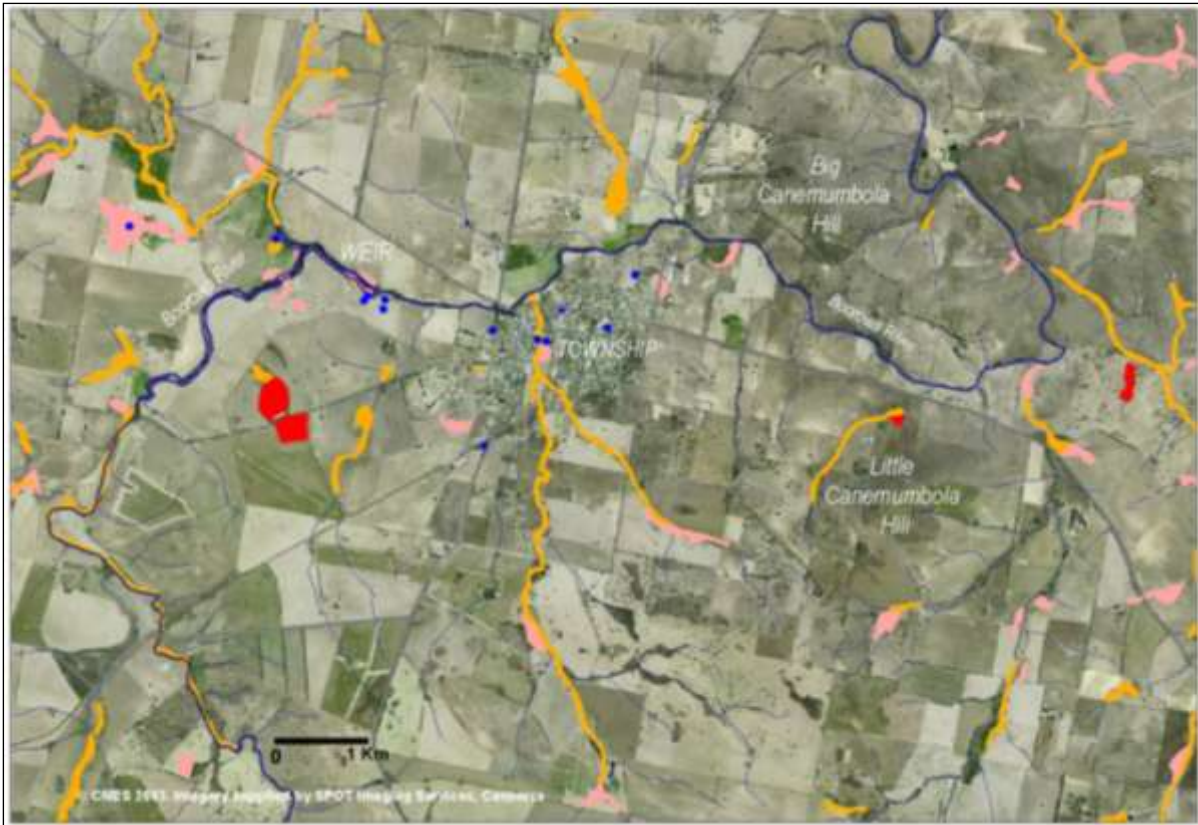
Figure 8 Dryland salinity occurrences in the vicinity of the Boorowa Township: orange - early phase of dryland salinity; pink – low- to moderate; red - severe salinity; blue circles location of groundwater monitoring piezometers (from DIPNR, 2002)
